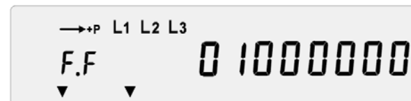
Figure 58. Example of an error message (insufficient battery voltage)
