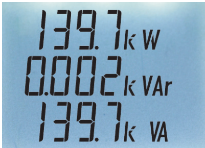
Active power Reactive power Apparent power
