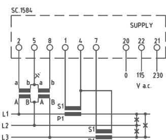
per linee trifase a 3 fili - for three-phase 3 wires system
