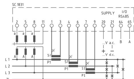
per linee trifase a 4 fili - for three-phase 4 wires system
